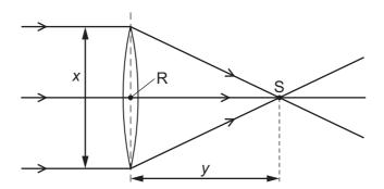
Which labelled point is the principal focus of the lens, and which labelled distance is the focal length of the lens?
